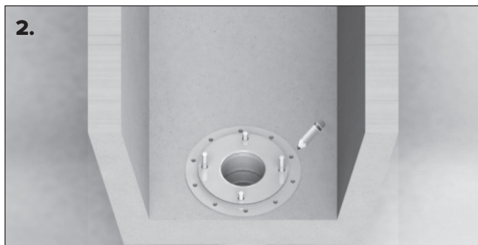
2. Insert outlet and mark area covered by outlet and holes for knock in plugs.
