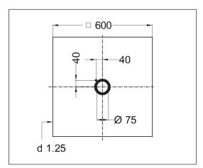
For a vapour sealed installation of the Akasison XL75 in metal roofs. Includes a metal reinforcing plate and rubber connection.
