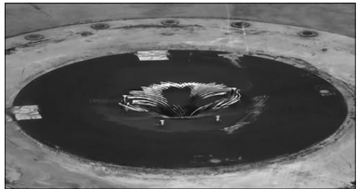
(a) no disc or airbaffle, large vortex.
